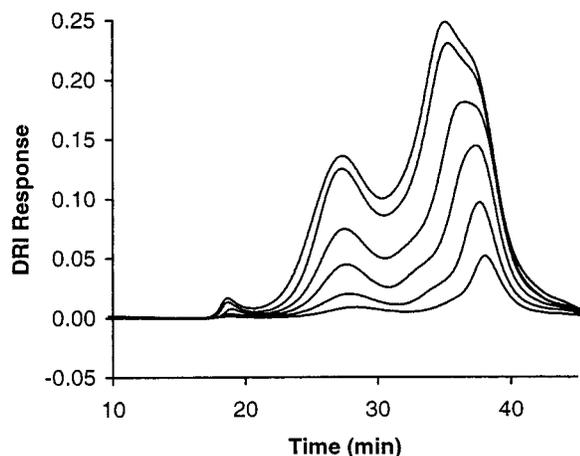
**Figure 8.** SEC-DRI elution profiles for a commercial sodium caseinate sample as a function of protein concentration: (a) 0.5, (b) 1.0, (c) 2.0, (d) 3, (e) 4, and (f) 5.0%.
