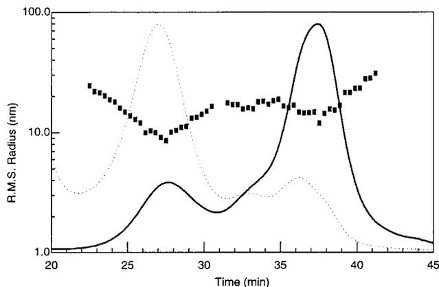
**Figure 6.** Plot of log z-average root-mean-square radius ( $R_g$ ) as a function of time (■) obtained for a 2% commercial sodium caseinate solution that had been ultracentrifuged. The elution profile is overlaid with the DRI signal (—) and MALLS at the 90° angle (···).
