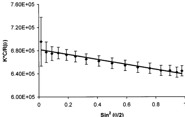
**Figure 5.** Debye plot showing the extrapolation of  $K^*c/R\theta$  to zero angle. The data shown correspond to a slice at 24.8 min in the data for 2% commercial sodium caseinate shown in Figure 4. The extrapolated value for  $K^*c/R\theta$  corresponds to a weight-average molar mass ( $M_w$ ) of  $(6.756 \pm 0.185) \times 10^5$  (g/mol), and the slope of the line shown yields a z-average root-mean-square radius ( $R_g$ ) value of  $14.9 \pm 0.4$  nm.
