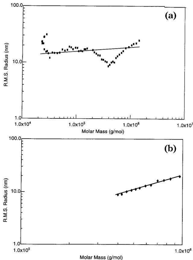
**Figure 7.** Plot of log z-average root-mean-square radius ( $R_g$ ) as a function of log molar mass obtained for a 2% commercial sodium caseinate solution that had been ultracentrifuged (a) the complete SEC-DRI spectrum and (b) the molar mass fraction between 400 and 970 kDa. The slopes of the regression lines for (a) and (b) were 0.07 ( $\pm 0.01$ ) and 0.91 ( $\pm 0.01$ ), respectively.
