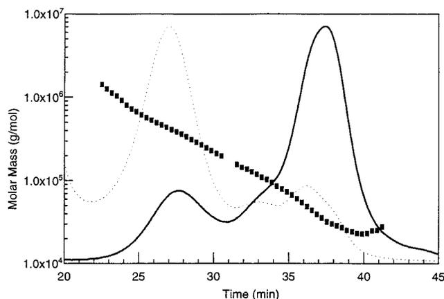
**Figure 4.** SEC-DRI elution profiles (—) of peaks 2 and 3 obtained for a 2% commercial sodium caseinate solution that had been ultracentrifuged. The elution profile is overlaid with the calculated molar mass (■) and MALLS at the 90° angle (···).
