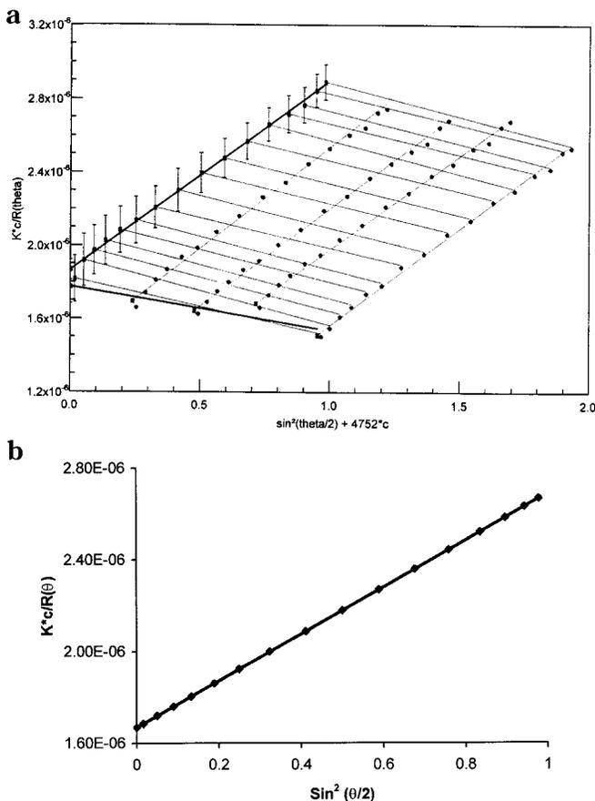
**Figure 1.** Zimm plot for a commercial sodium caseinate sample (ultracentrifuged), which had a z-average root-mean-square radius ( $R_g$ ) of  $48.7 \pm 2.1$  and weight-average molar mass ( $M_w$ ) of  $(5.493 \pm 0.334) \times 10^5$  (g/mol) (a) and an example of a Debye plot calculated from one of the concentrations used to make this Zimm plot, which yielded an  $R_g$  value of  $51.2 \pm 0.3$  nm and a  $M_w$  of  $(5.993 \pm 0.029) \times 10^5$  (g/mol) (b).
